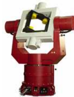
Figure 1. Flight simulation with six-degrees of freedom.
